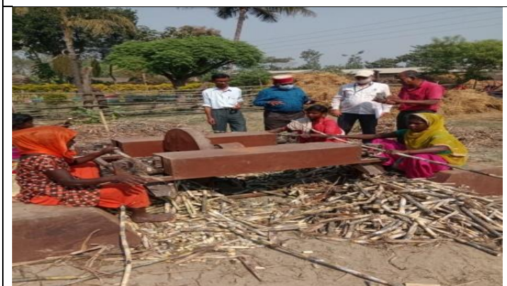
Modified electric power sugarcane bud cutter and hand sugarcane bud cutter
