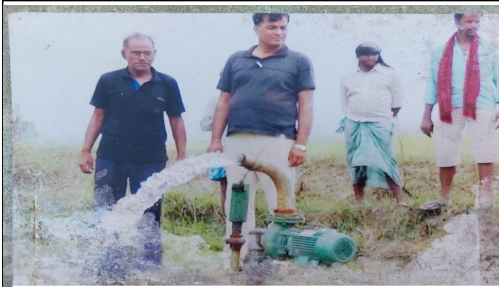
PTO. (Power Take-off) - tractor driven generator operate at a time 3-4 tube wells simultaneously for irrigation in the area of Gandak basin (within 1 kilometer radius)
