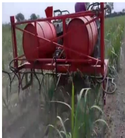
Modified boom sprayer-tractor operated and modified knapsack sprayer
