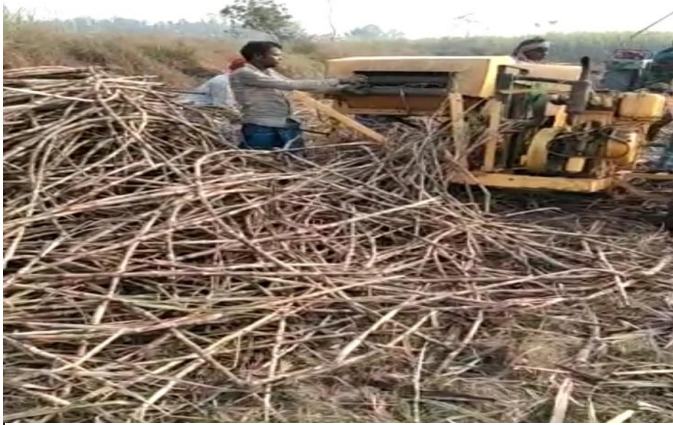
Modified sugarcane leaf destresser machine with 5 HP engine-suitable for slicing all types of sugarcane easily at low cost and in less time
